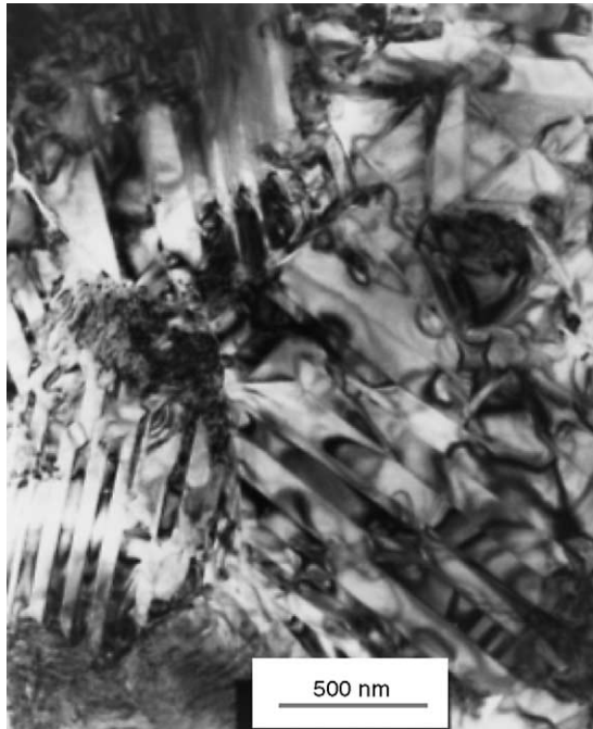
Fig. 4. TEM micrograph of the 8 mol% CeO 2 stabilized ZrO 2 ceramic sintered by SPS.
