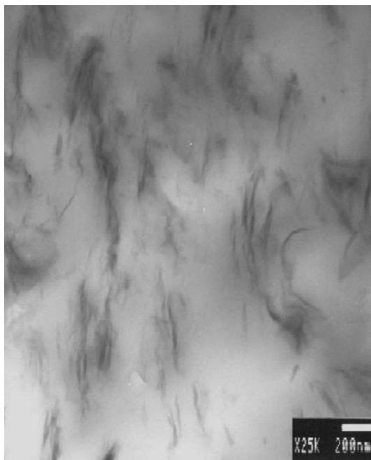
Fig. 1. Structure of polypropylene/5% organo-montmorillonite composite (fabricated by CAOL + ICSI, Haifa); TEM, bright field image showing partially and, some, fully exfoliated OM tactoids (black filaments).
